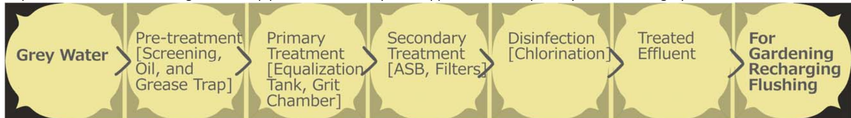
Figure 12 | The on-site filtration sequence for grey water.
